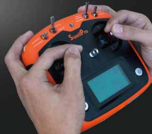
It is easy to find your lost drone with buzzer alarm by pressing the buttons on the backside of the controller. Arming or disarming the motors is now triggered with a switch, which shortens startup time and prevents accidents.
