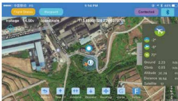
8. **Point-to-Fly:** Click the “Point-to-Fly” button, and then click the target point on the map, the drone will start flying to the point and hover there.
