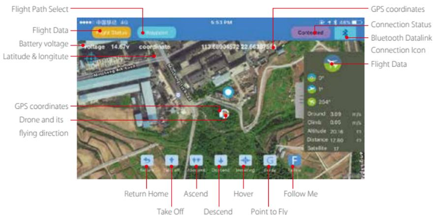
4. Once you have a minimum of 9 GPS satellites, you can unlock the drone and start flying with controller, or use the APP to unlock the motors and start flying.
